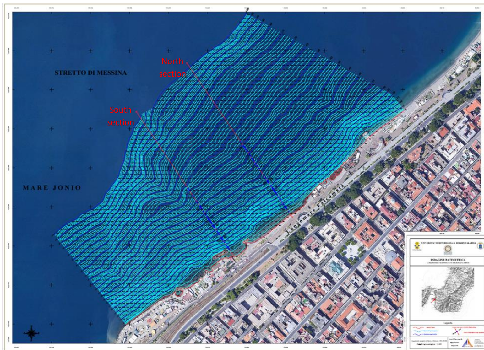
Figure 12. Bathymetry survey at NOEL site. The red lines orthogonal to the shoreline indicated the two transects chosen to draw the bottom profile reported in Figure 13.
