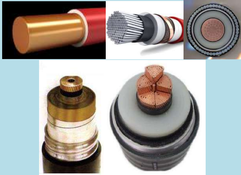
From upper left to bottom right: solid, stranded, profiled, hollow, milliken
