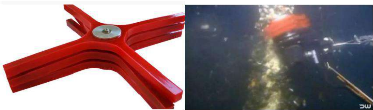
Figure 29. ROV based technology for biofouling removal from submerged surfaces
