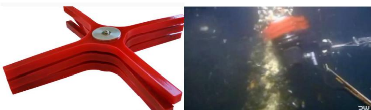
Figure 2-27. ROV based technology for biofouling removal from submerged surfaces
